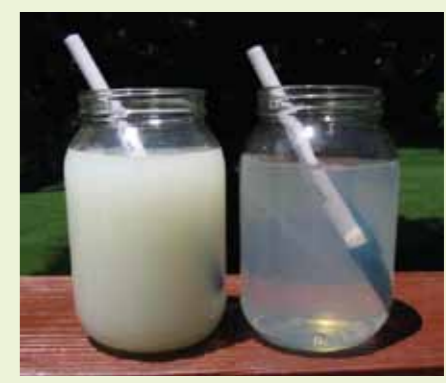
Solvent-based clear coat system water treated with conventional based chemistry programmes (left). Same clear coat treated with APEX programme (right).
